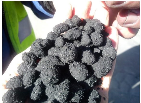
One type of active capping material, AC-amended BioBlok® (source: BioBlok Solutions AS).
