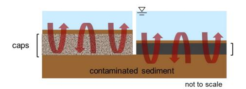
As for isolation capping, other factors including possible groundwater upwelling, geotechnical stability, and ebullition also need to be considered when designing and constructing conventional or active thin-layer caps
