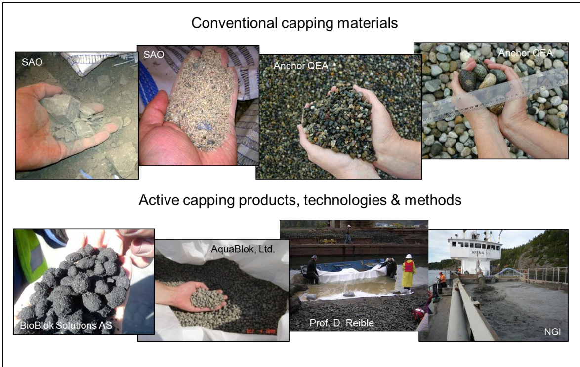
Figure 3.4 Conventional and active capping materials, products and technologies (photo sources provided).
